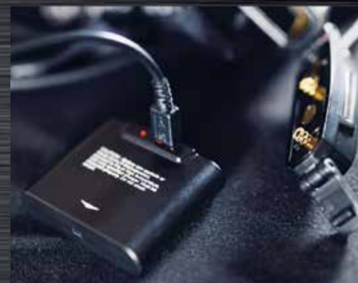
Removable battery pack with charging indicator
