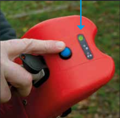
Floodlight can be operated from ground level switch
