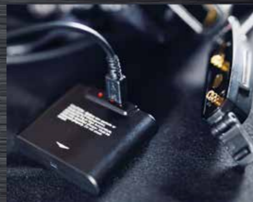
Removable battery pack with charging indicator
