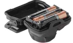
Lift the open launch on top of the head torch and pull open the battery compartment. Insert 3 x AAA alkaline batteries into the battery compartment.
