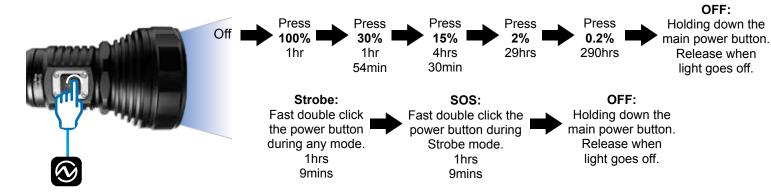
Memory Function: Flashlight will remember the last mode that was being used before being switched OFF and return to this mode when switched back ON.
