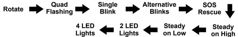
To turn off the warning light without cycling through the 9 light modes, press and hold the power button for 2 seconds. Two LEDs will flash five times and then turn off. When ready to operate again, press the power button once and it will return to the last flash mode that was selected before turning off.
